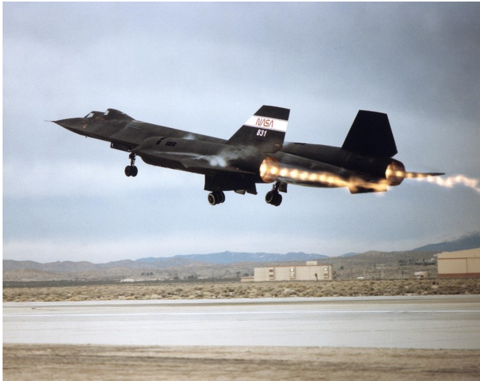
Figure 4.5: The Lockheed SR-71 with visible Mach disks due to an overexpanded jet (from [NASe]).
